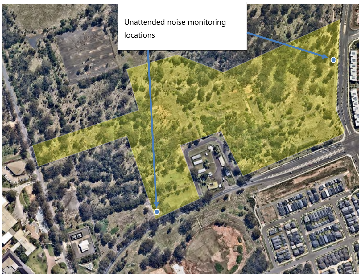
Figure 3 - Aerial view of site showing long term unattended noise monitoring locations
